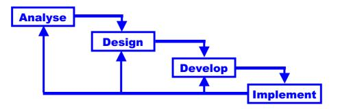
This model attempts to overcome the limitations of the original Waterfall Model by adding an "iterative" loop to the end of the cycle. That is, in order to keep up with changing requirements the "analysis" phase is revisited at the end of the cycle and the process starts over again.
