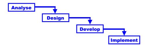
The Waterfall Model was widely adopted in the early days of software development and a lot of blame has been laid at its door. The model was derived from engineering models and while it does prove a useful point it is intrinsically flawed.
