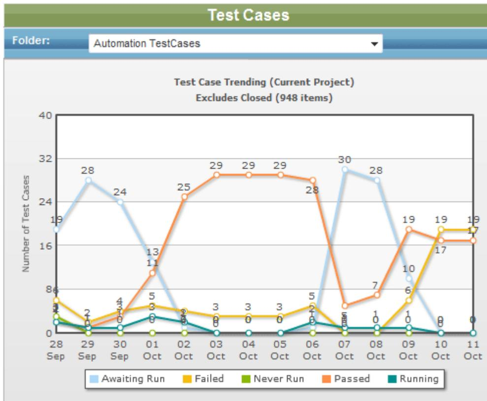
As you can see from the graph above, the past 2 days (Oct 10/11) has introduced a problem in the code because 19 automated test cases failed while 17 passed. Looking at the graph, you can see that the the issue was introduced on Oct 9, as all test cases passed from Oct 2 - Oct 6. This type of information is invaluable for quality assurance teams.
