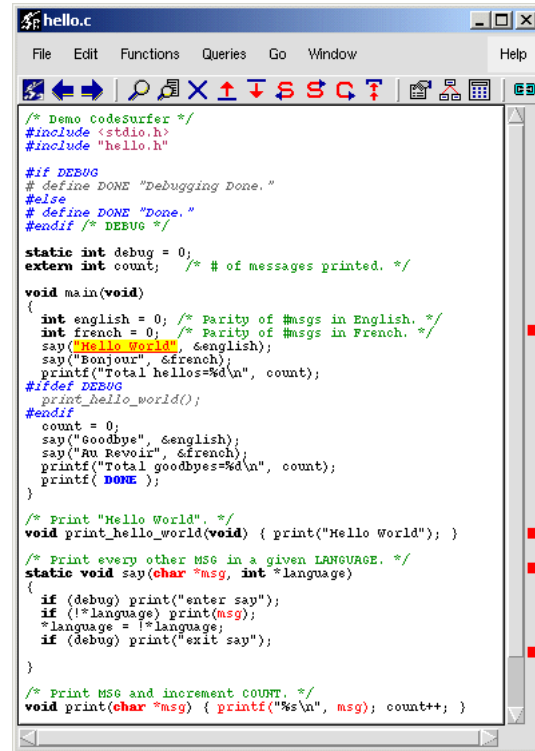
Fig. 4. A File Viewer for a small program. In this example, the user has selected the first parameter to the first call to the procedure say , and has invoked a forward slice query. All points that depend on this parameter are shown in red
