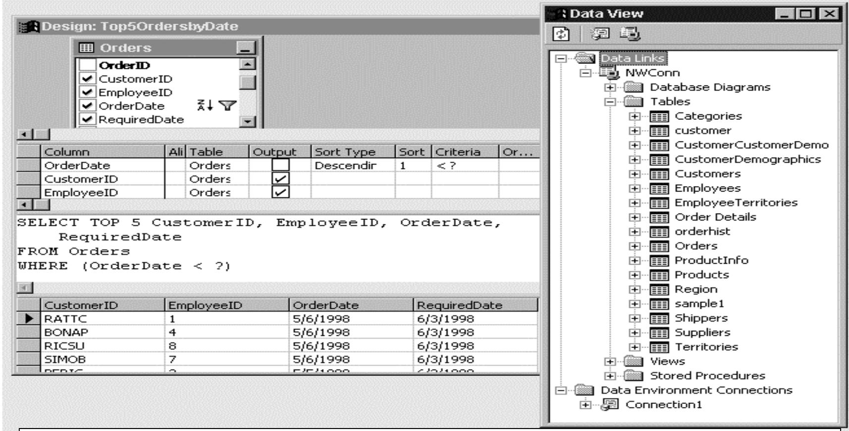
Figure 1. The Visual Data Tools windows include the Data View window for linking to a database and the Query Design window for creating and testing SQL statements.
