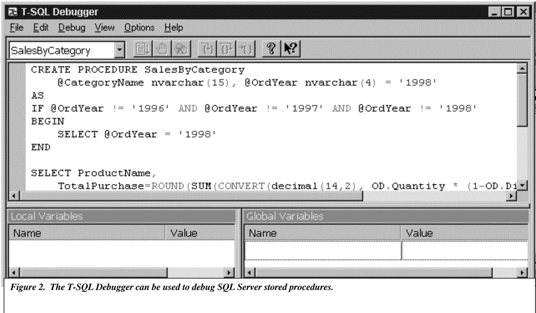
Figure 2. The T-SQL Debugger can be used to debug SQL Server stored procedures.
