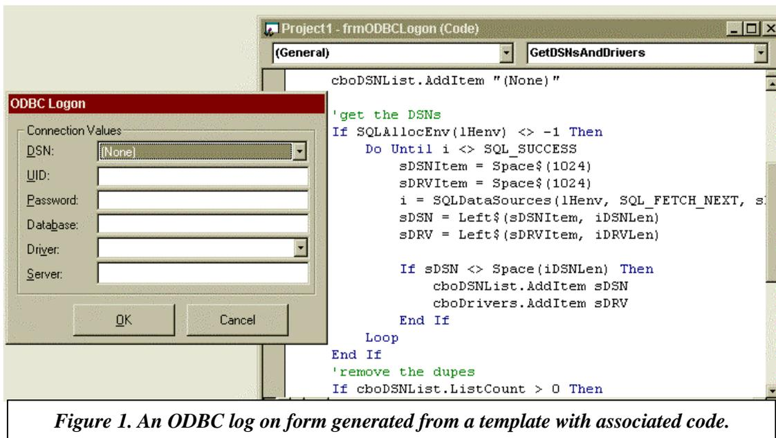
*Figure 1. An ODBC log on form generated from a template with associated code.*
