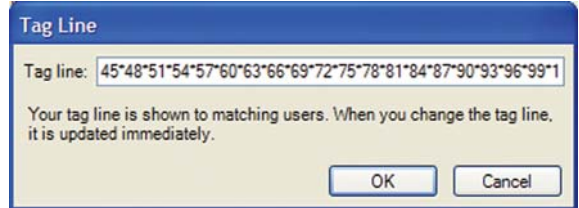
Figure 1: Using a counterstring to test the Tag Line feature in the Windows version of my client's application
