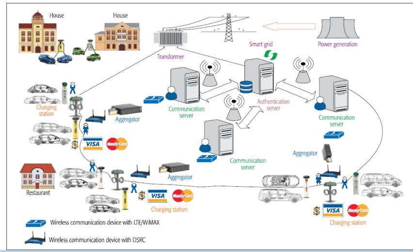
The V2G network has a higher level of scale and complexity:
